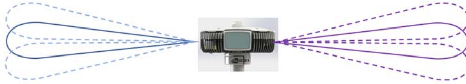
Figure 3: Vertical adjustment of the Pandora360 Radio Lobe.
