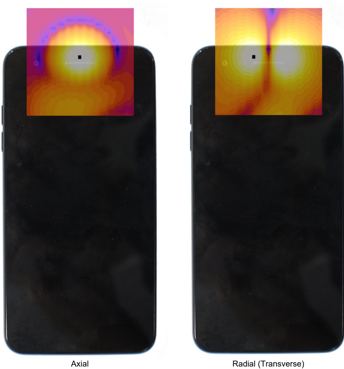
Axial Radial (Transverse) Figure 15-3 T-Coil Scan Overlay Magnetic Field Distributions
