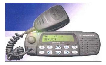
The CDM1550 LS, model PMUD1765A is a mobile transceiver that operates on trunked LTR (a transmission based trunking protocol for single site trunking) and Passport systems (an enhanced trunking protocol for wide area dispatch) as well as on conventional (single channel unit to unit communications) radio systems. The intended use of the radio is Push-To-Talk (PTT) while the device is properly installed in a vehicle with an external antenna mounted at the center of the roof or trunk.
