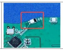
The antenna is Chip antenna.
