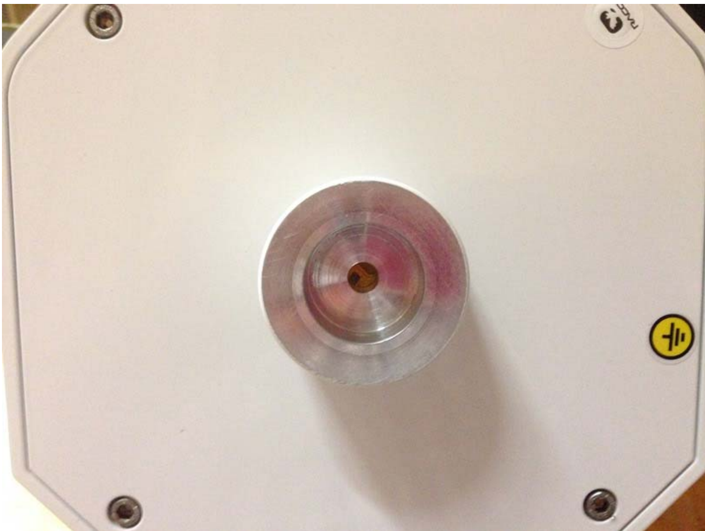
Side 2 of 6, Detail of Waveguide Port
