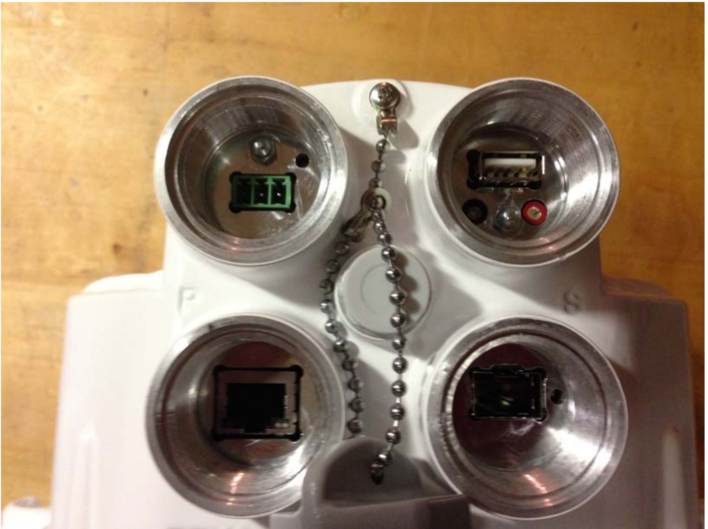
Side 5 of 6, Detail of I/O and Power Ports
