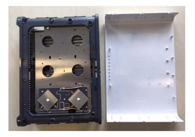
Photograph No.2 "AirUnity 545 eNB 2.5 GHz (B41)" station internal view, rear side
