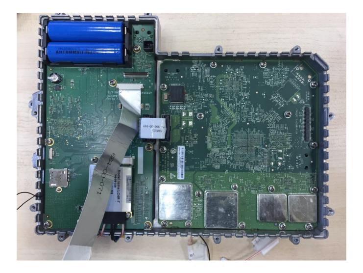
Photograph No.5 "AirUnity 545 eNB 2.5 GHz (B41)" station internal view
