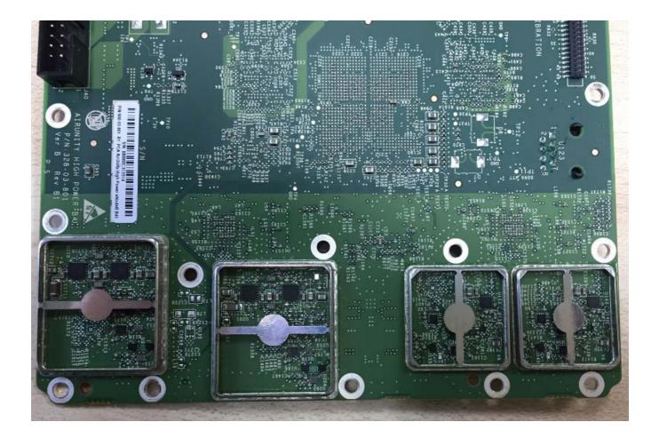
Photograph No.7 Main board close view with shields removed
