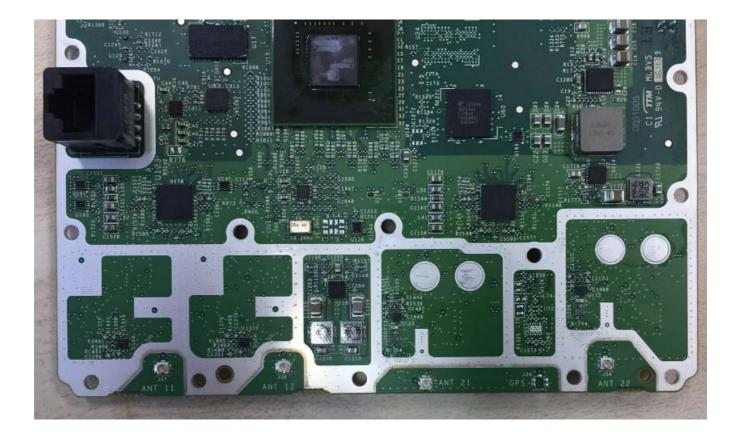
Photograph No.9 Main board second side close view, antenna connectors
