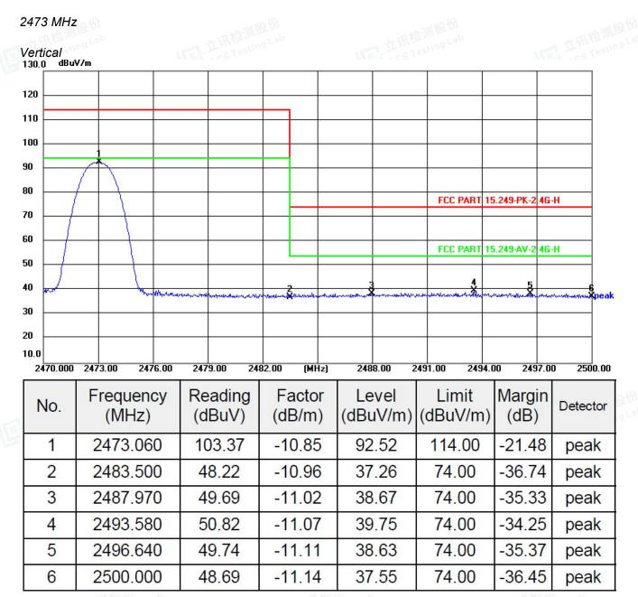
Note: Due to the measure PK emission level less than the AV limit value. No necessary to take down the AV emission level.
