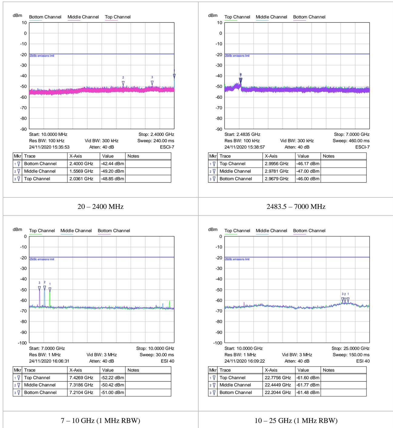
Figure 4: Emissions in non-restricted frequency bands
