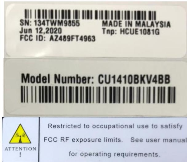
Figure 2: FCC Label for CU1410BKV4BB (CLS1410)
