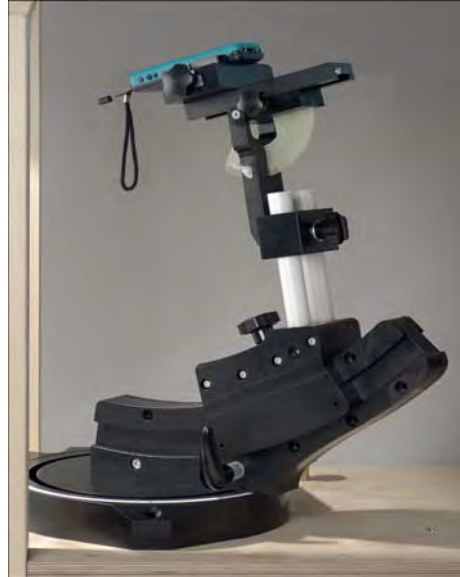
F-2. Device Holder for Transmitters
