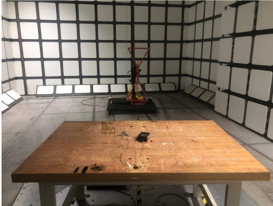
Radiated Emissions View (Below 1 GHz)
