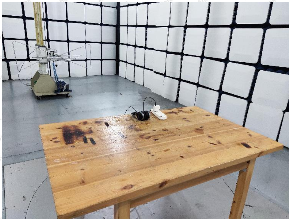
Photo of Radiation Emission Test
