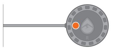
There is a smaller button located next to the Multi-Function Button on both earpieces. With it, you can either disconnect from your Bluetooth device or clear the memory of the Pucks 2.
