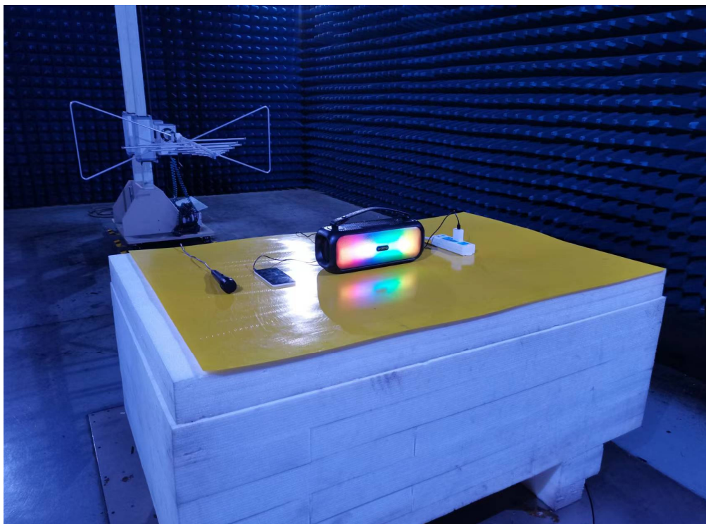
Photo of Radiated Emission Measurement (Above 1G)
