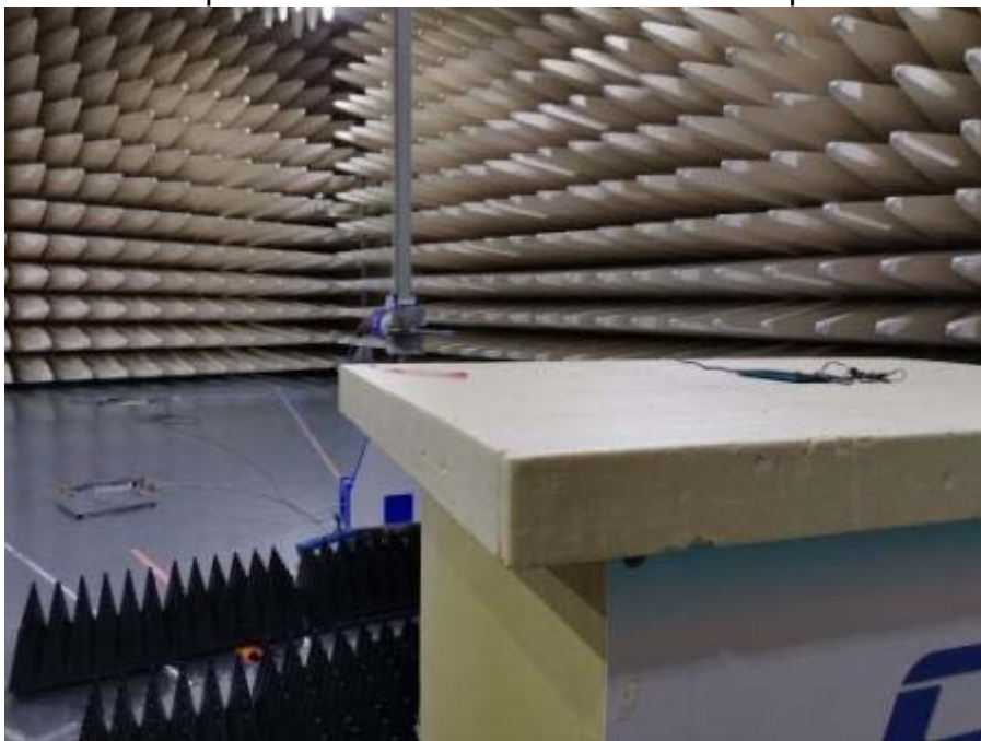
Spurious Radiated Emissions Test setup
