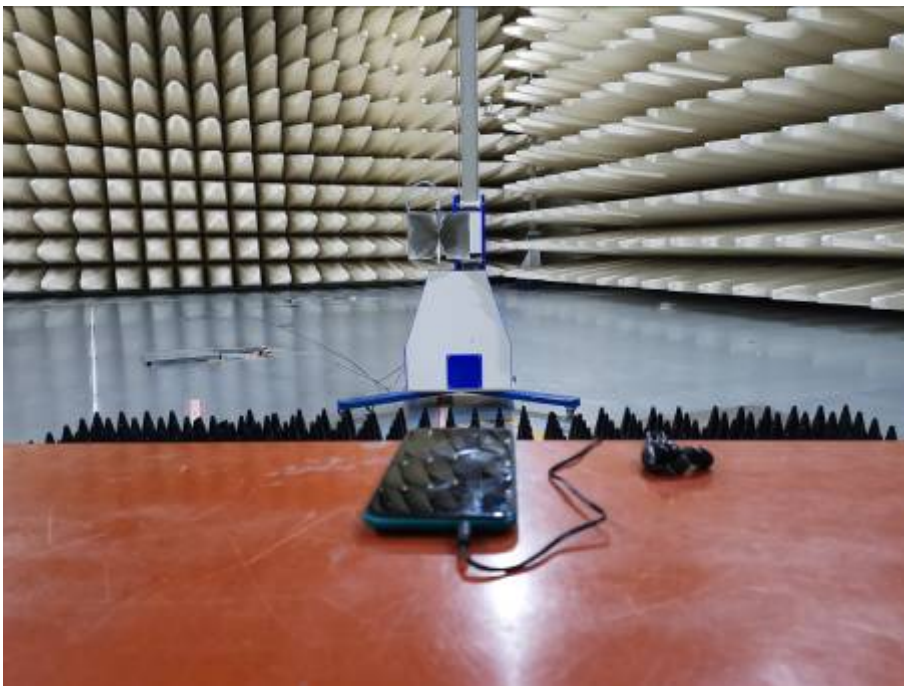
Radiated Emissions Test Setup (above 1GHz)
