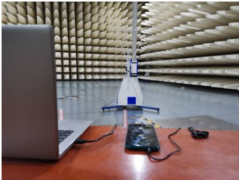
Radiated Emissions Test Setup (30-1000MHz)
