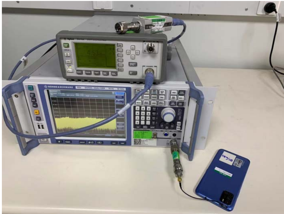
RF Conducted Test setup (BT/BLE/WIFI)
