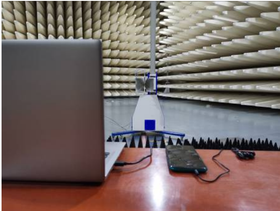
Radiated Emissions Test Setup (above 1GHz)
