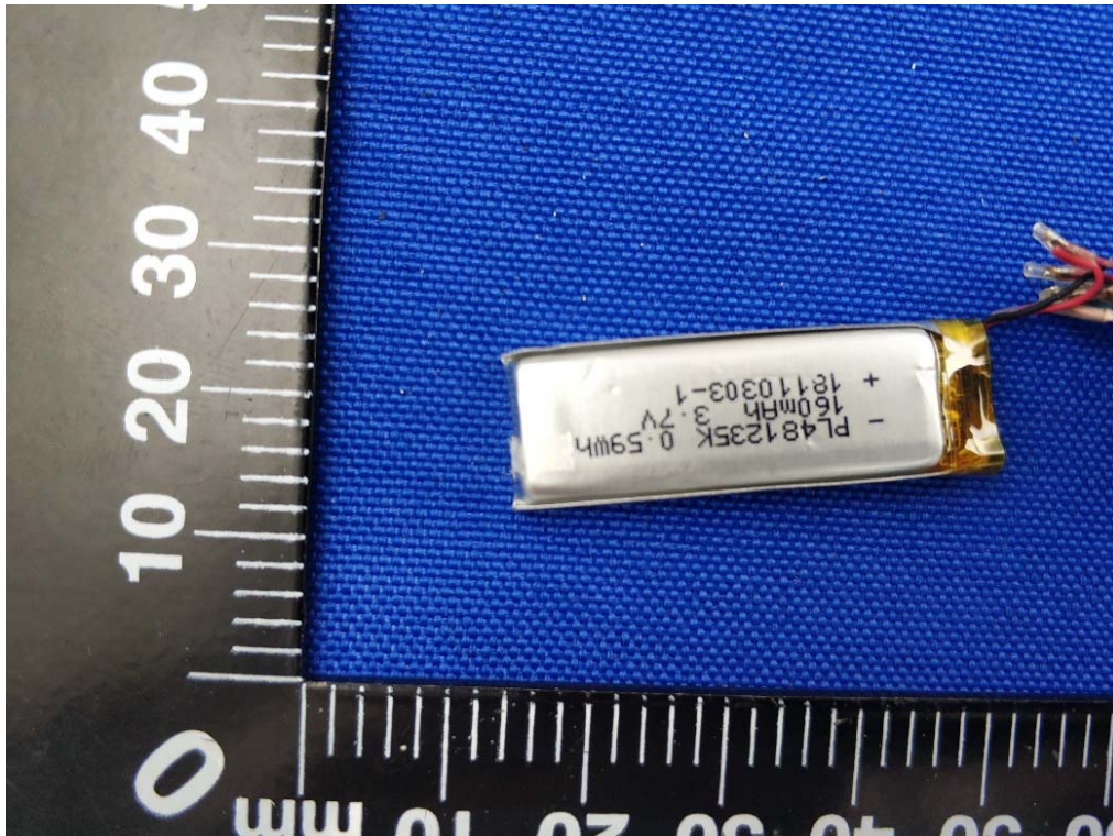
Battery Photo (FRONT)
