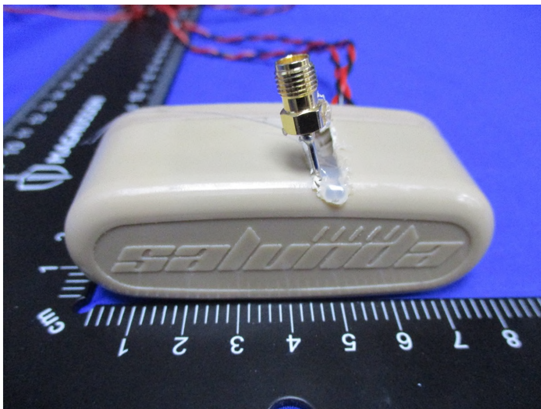
Conducted sample with temporary antenna port
