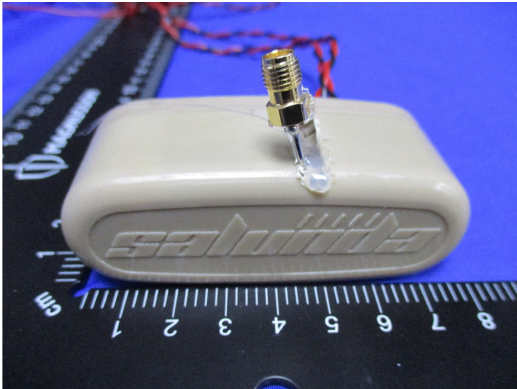
Conducted sample with temporary ZigBee antenna port
