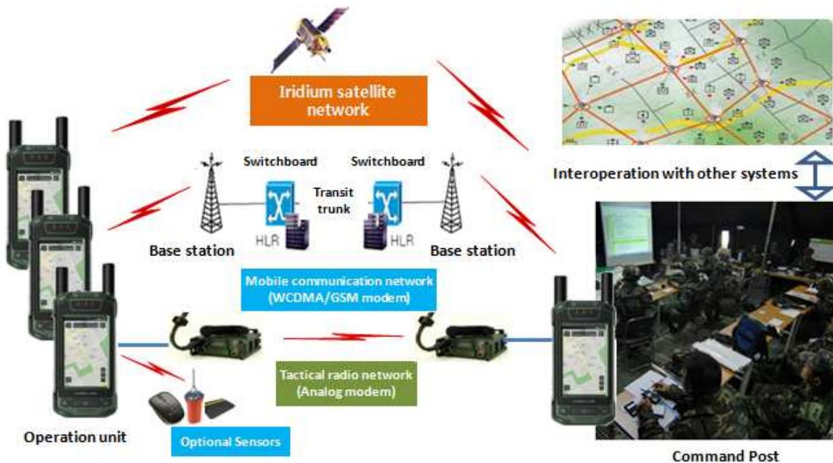
Figure 1-1 operational diagram of mBFT17
