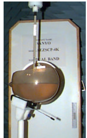
Fig. 1 SAR Test Set-up
