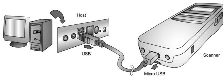
Insert the Micro USB connector into the port on the scanner and the standard USB connector of the USB cable into a USB port on the host PC.
