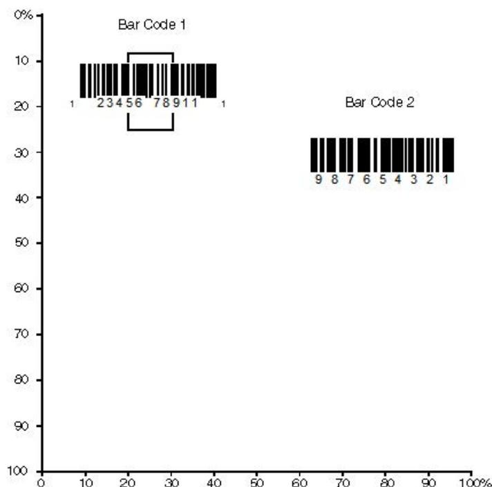
Scan Presentation Centering On, then scan one of the following bar codes to change the top, bottom, left, or right of the centering window. Then scan the percent you want to shift the centering window using digits on the inside back cover of this manual. Scan Save. Default Presentation Centering = 40% for Top and Left, 60% for Bottom and Right.
