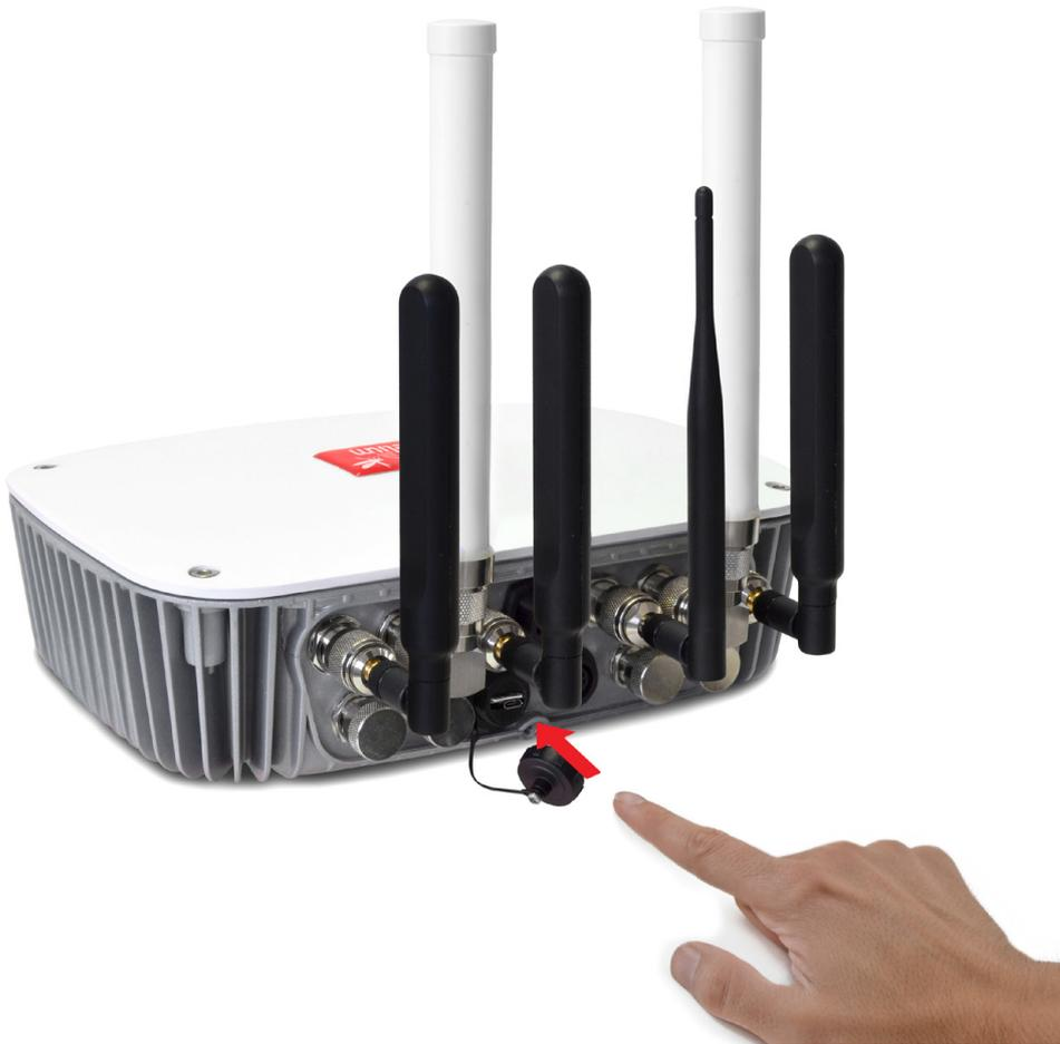
Figure : Inserting a SIM card with care in the External SIM socket
