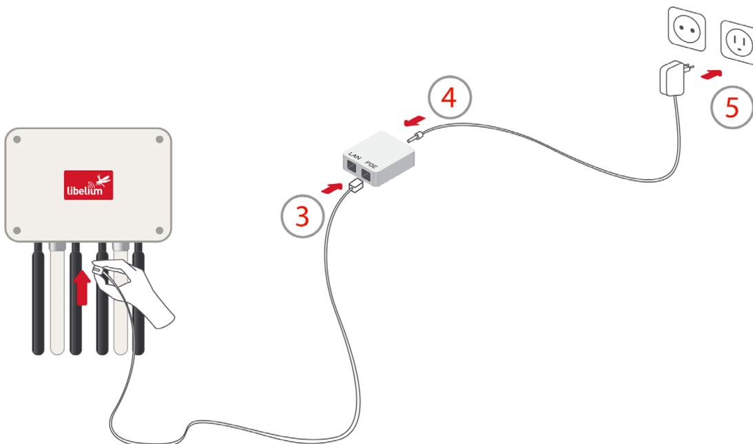
Figure : How to connect Meshlium to 220V
