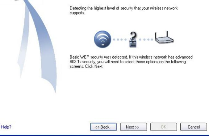
6. Select the **Network Authentication** and **Data Encryption** options. Enter the encryption key settings and configure the 802.1x settings as required. Refer to <u>Security Settings</u> for more information.
