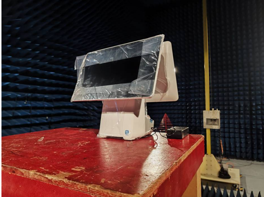
Radiated Test Setup Photograph(HK528 (second display:15.6 inch))
