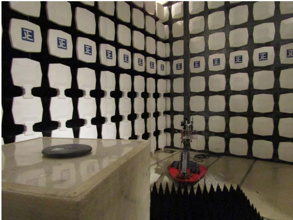
Measurement of Radiated Emission Test Set Up
