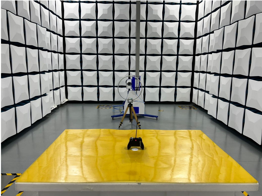
Set-up of Radiation Emission below 30MHz
