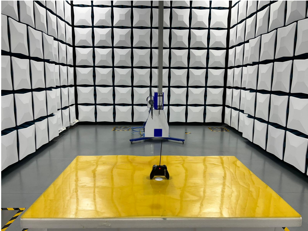
Set-up of Radiation Emission from 200 – 1000MHz
