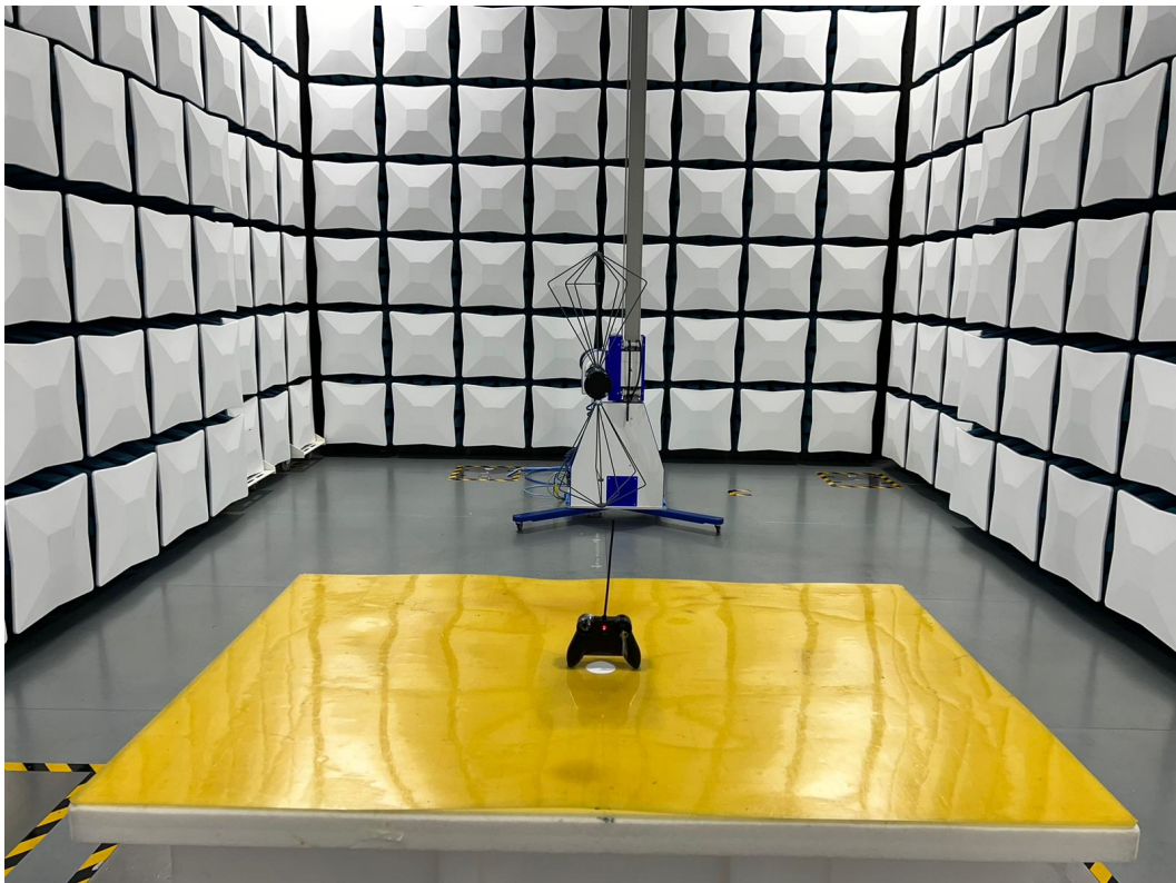
Set-up of Radiation Emission from 30 – 200MHz
