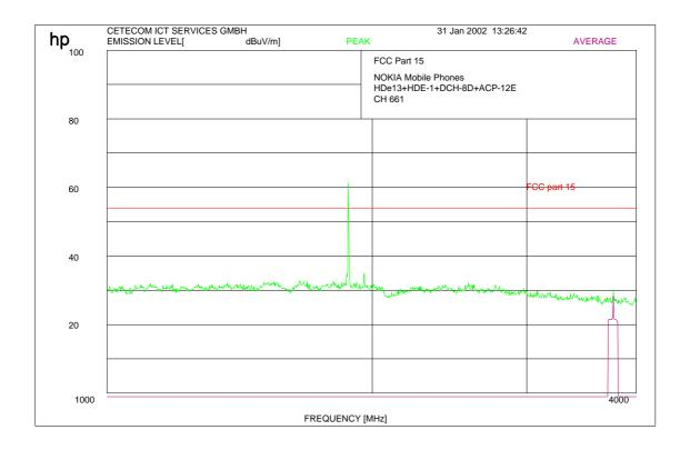
3763.5 MHz  $30.8 \text{ dB}\mu\text{V/m AV}$
