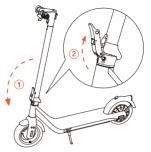
2. Unfold the stem and fasten the folding wrench. Make sure the unlocking key springs up normally after fastening. Be sure to buckle up properly.
