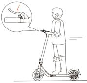
4. Slow down by releasing the throttle and hold the braking lever lightly (Do not brake suddenly and watch out for the road conditions!).
