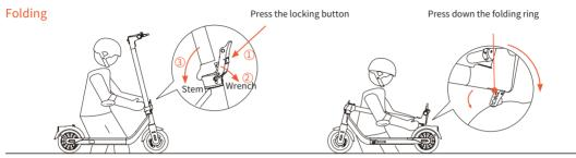
Power off the scooter, hold the stem, press the locking button and pull the lever, bend the handlebar stem towards the footrest. Hold the stem and pull the folding ring, attach the hook to the locking clip on the side of the mudguard.
