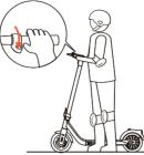
Do not press the throttle when walking with the scooter.
