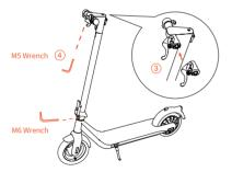
3. Place the brake lever on the handlebar,tighten it firmly with hex wrench to be sure it won't loosen. (Note: Use the M6 wrench to re-tight the folding part's nuts in case it's loosen after long time use)
