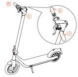
4. Install the handles on the stem and firmlya tighten it according to the correct position and direction marked on the label.
