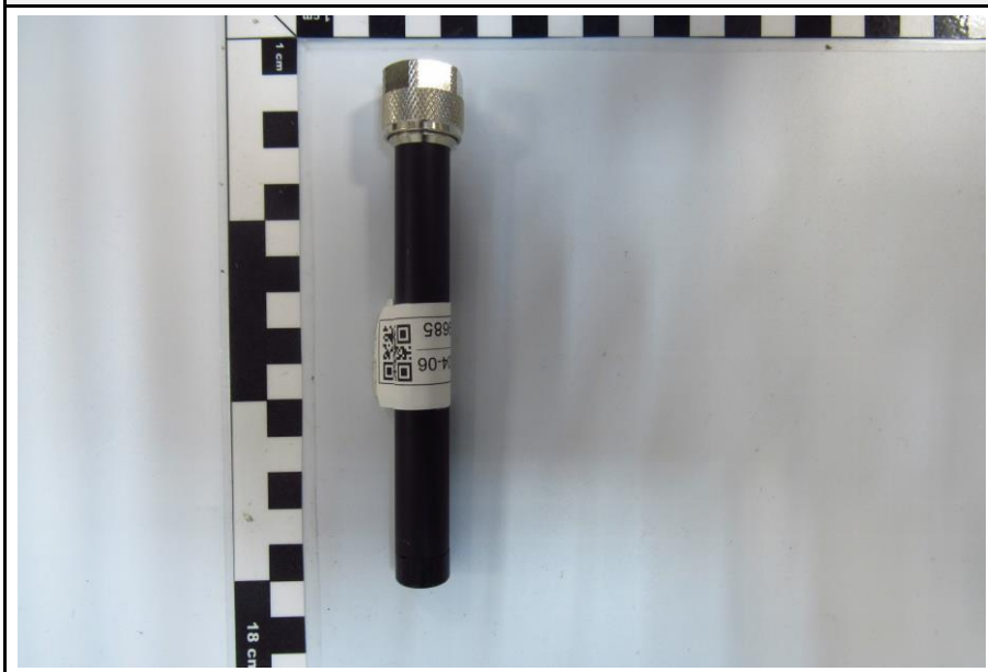
Ancillary equipment: Antenna F9915KW
