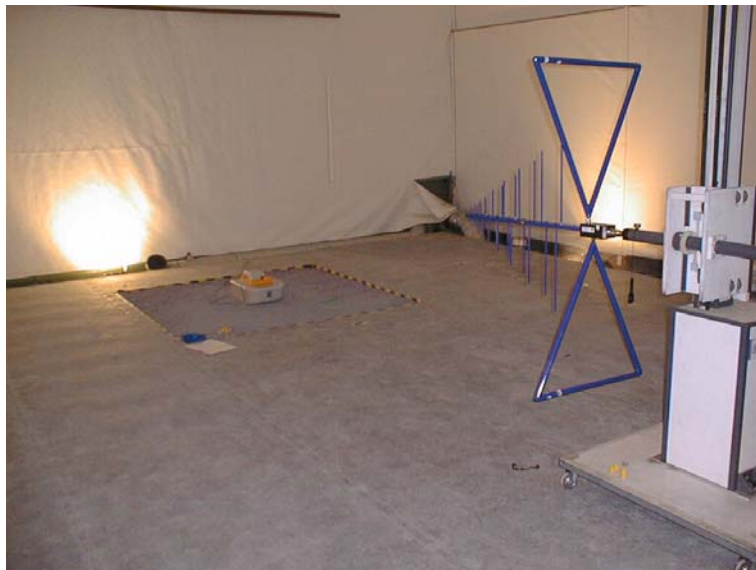
Picture 2: EUT setup on sand bed
