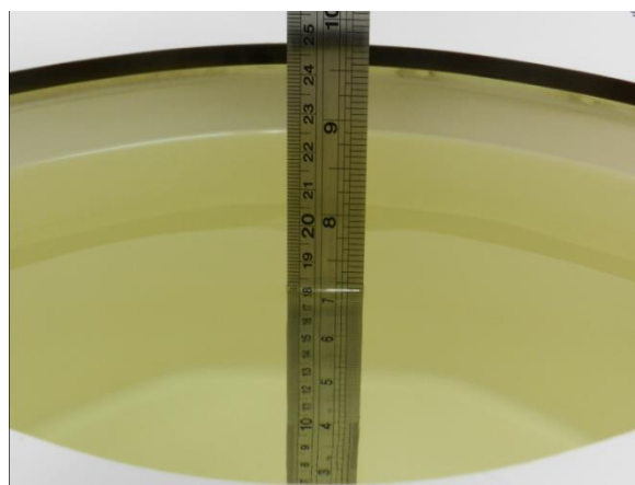
Fig 10.2 Photo of Liquid Height for Body SAR
