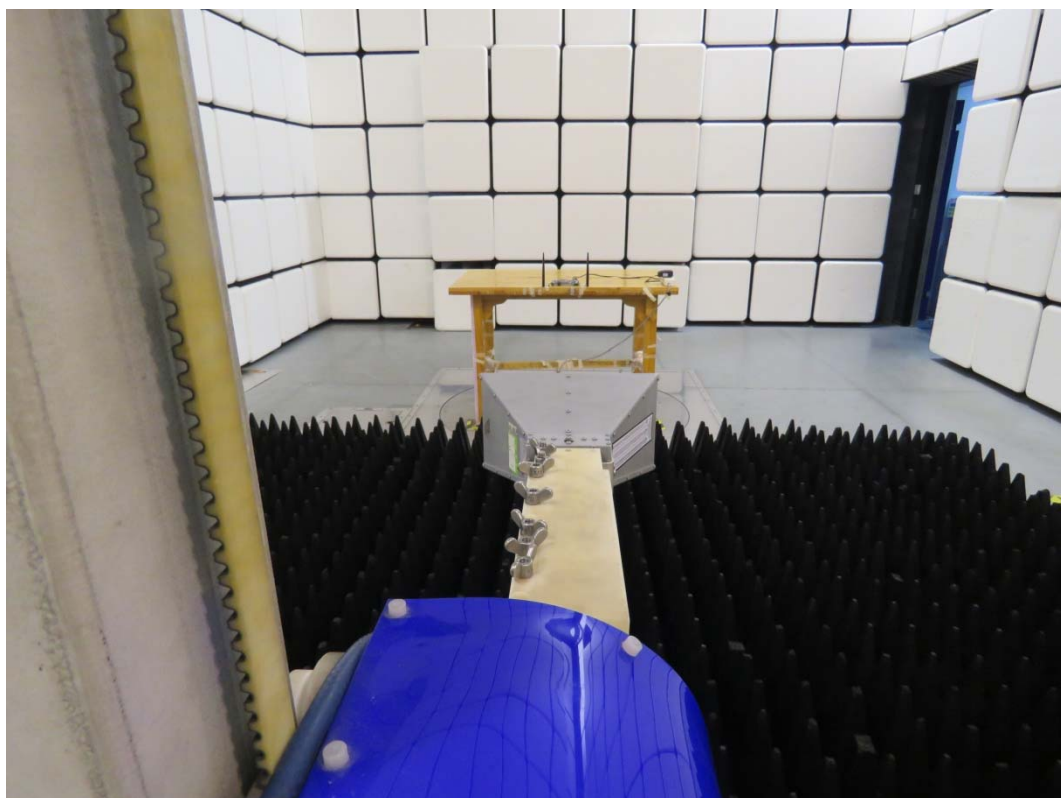
Picture 2: Radiated Spurious Emissions Test setup
