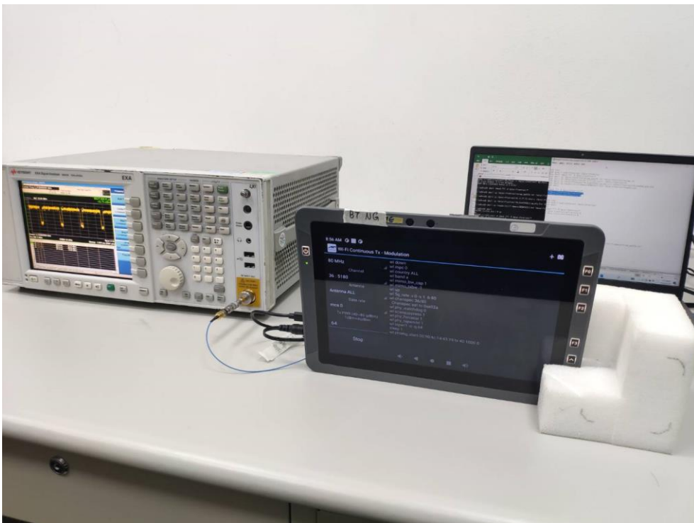
Description: Conducted Emission Test Setup
