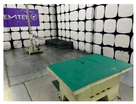
Spurious Emission Test Setup (Above 1GHz)
