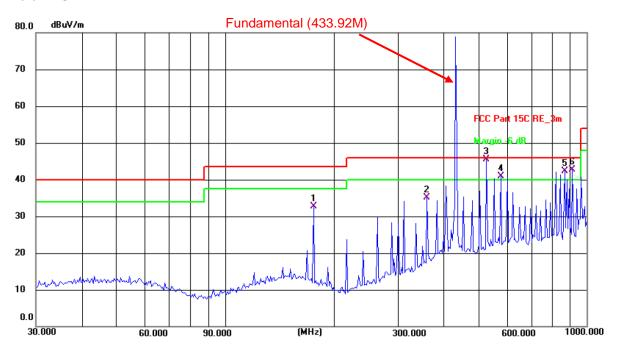
Site: 3m Anechoic Chamber Polarization: Horizontal Temperature: 24.3(C) Humidity: 50 %
