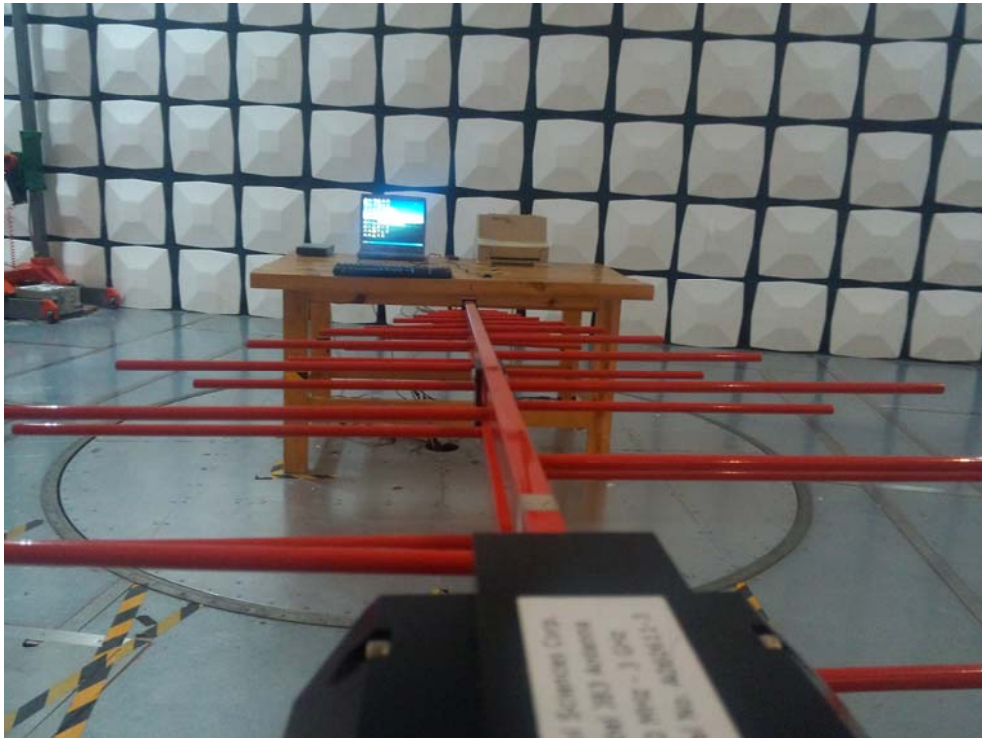
Radiated Emission Below 1GHz – Front View
