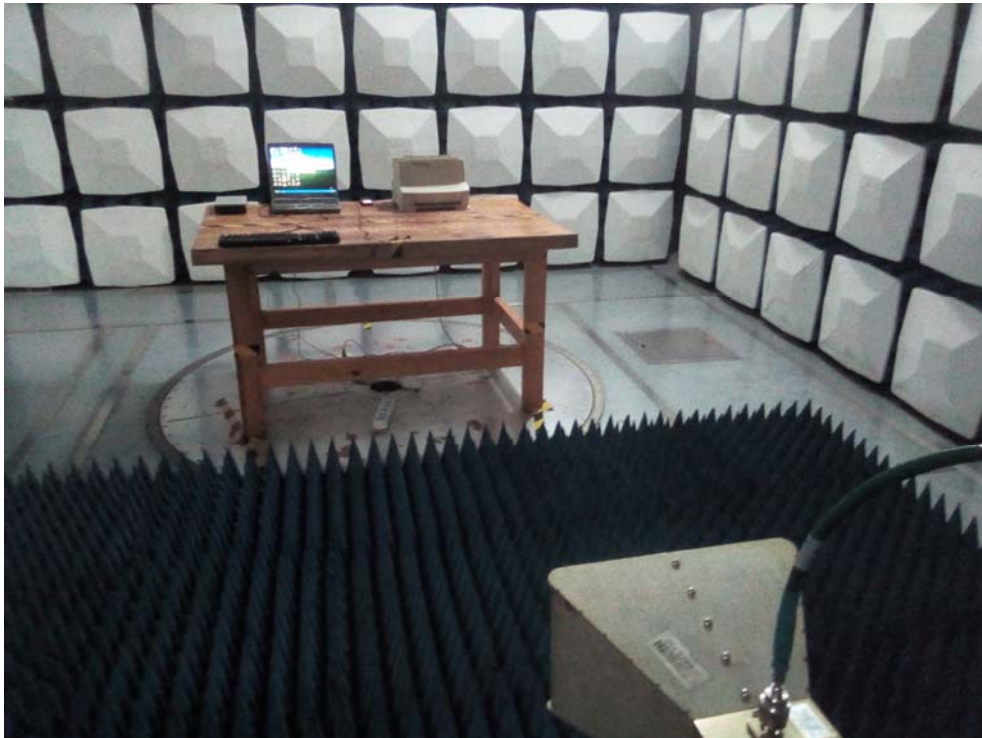
Radiated Emission Above 1GHz – Front View
