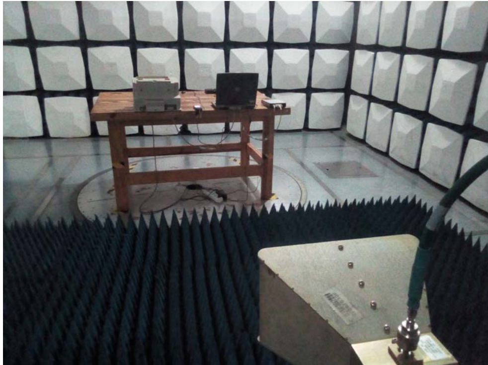
Radiated Emission Above 1GHz – Rear View
