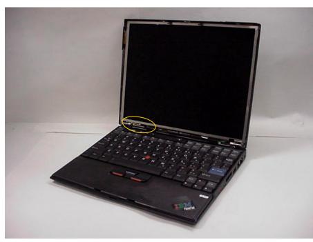
The main and auxiliary antennas located at LCD section of each host device (ThinkPad X30 Series, or X40 Series) are assembled apart from each Bluetooth antenna with 20 cm or more as shown in the previous pages.
