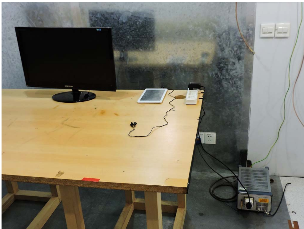
Conducted Emission Test Setup:
