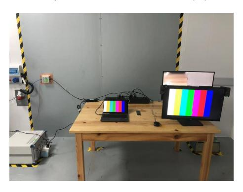
Set-up for Radiated Emission (RE), Below 1GHz
