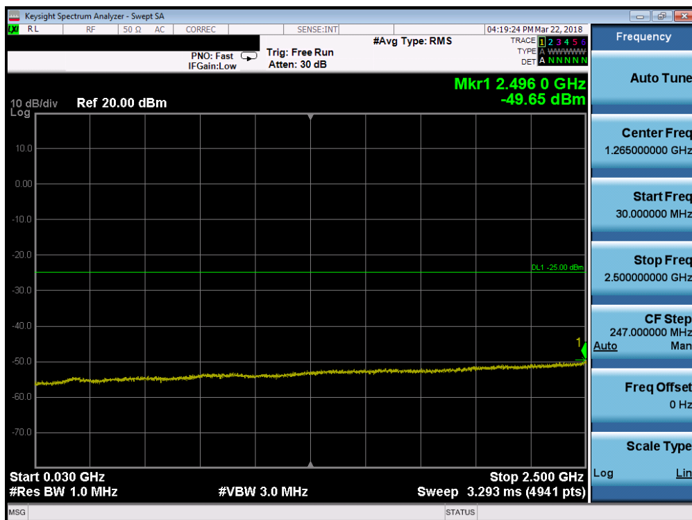
Plot 7-163. Conducted Spurious Plot (Band 7 - 5.0MHz QPSK - RB Size 1, RB Offset 0 - Mid Channel)
