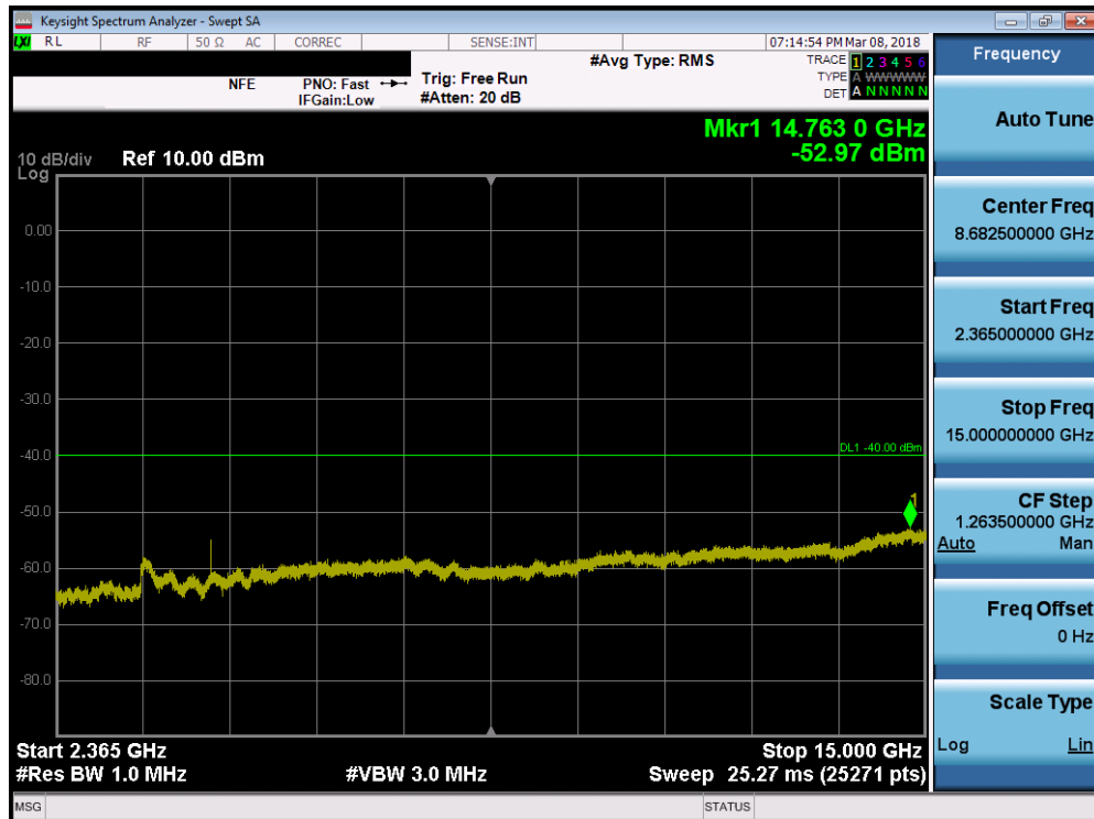
Plot 7-158. Conducted Spurious Plot (Band 30 - 10.0MHz QPSK - RB Size 1, RB Offset 0)
