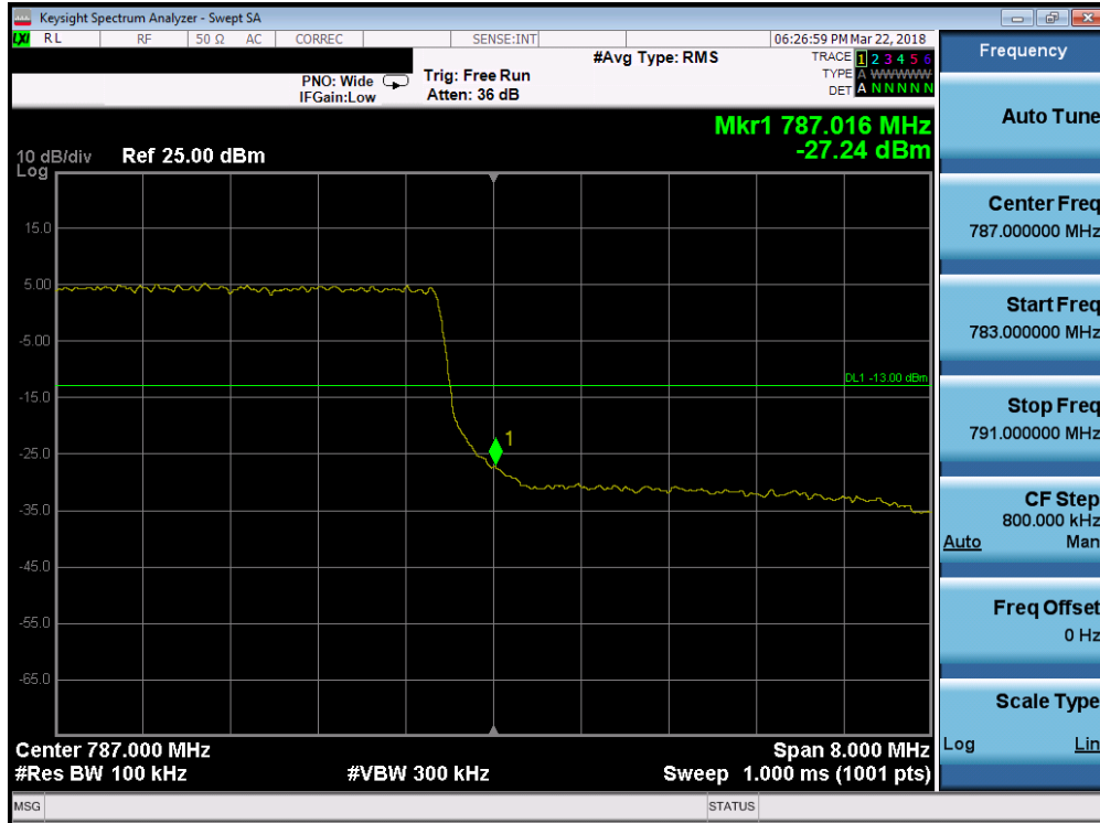
Plot 7-202. Upper Band Edge Plot (Band 13 - 10.0MHz QPSK - Full RB Configuration)
