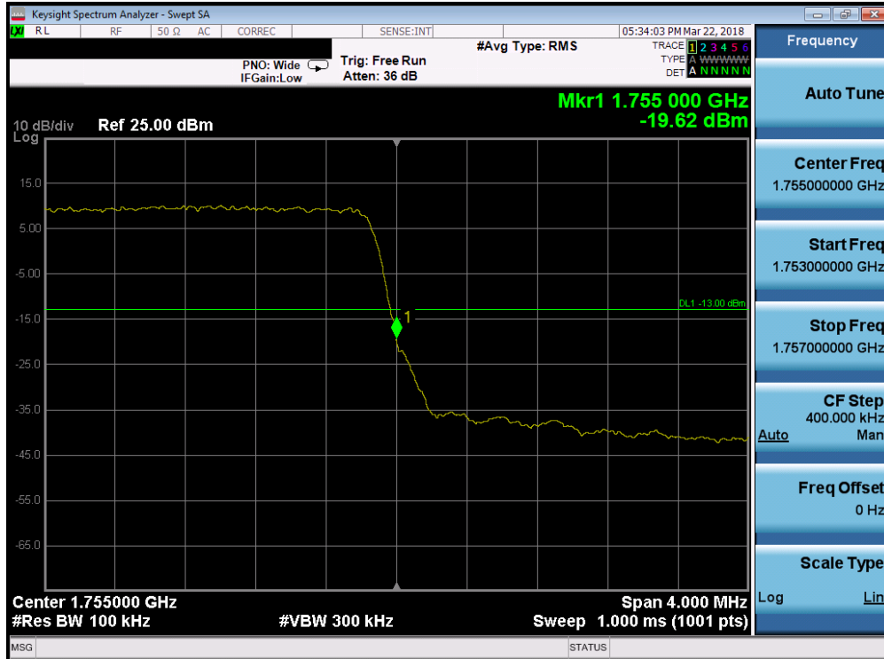
Plot 7-220. Upper Band Edge Plot (Band 4 - 3.0MHz QPSK - Full RB Configuration)
