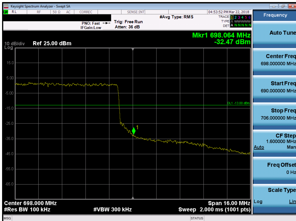
Plot 7-185. Upper Band Edge Plot (Band 71 - 20.0MHz QPSK - Full RB Configuration)
