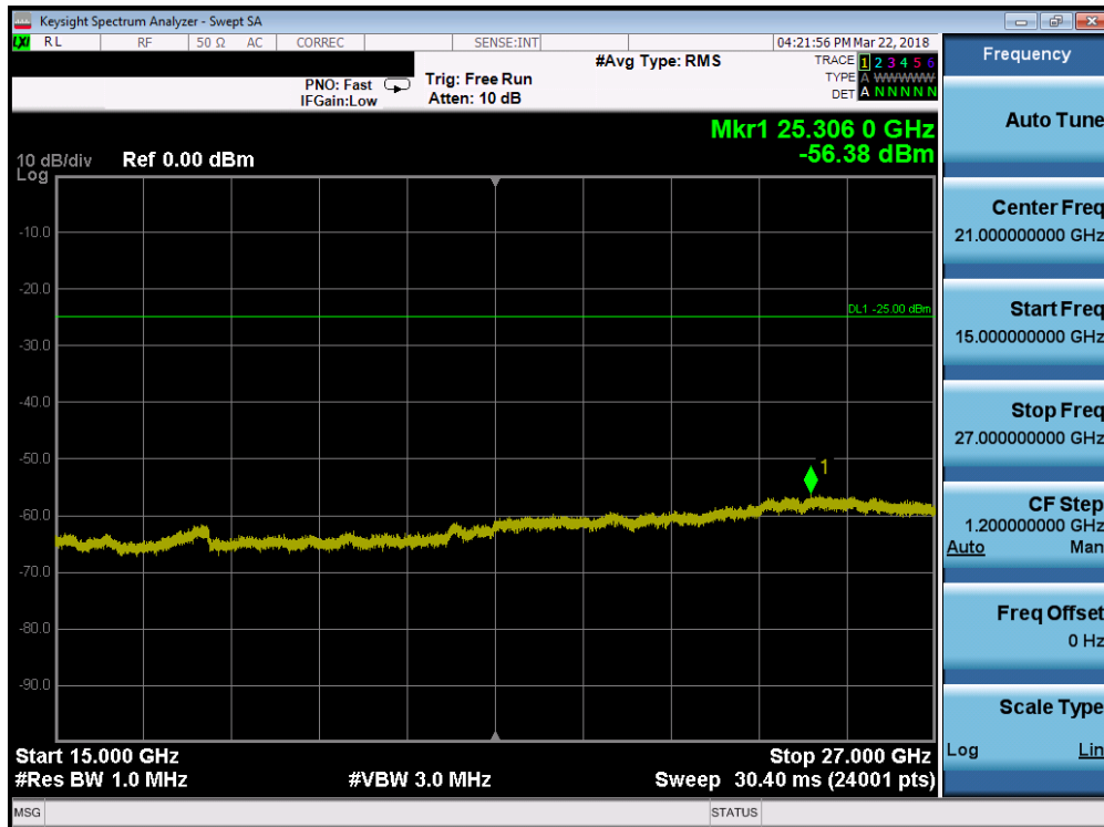
Plot 7-168. Conducted Spurious Plot (Band 7 - 5.0MHz QPSK - RB Size 1, RB Offset 0 - High Channel)
