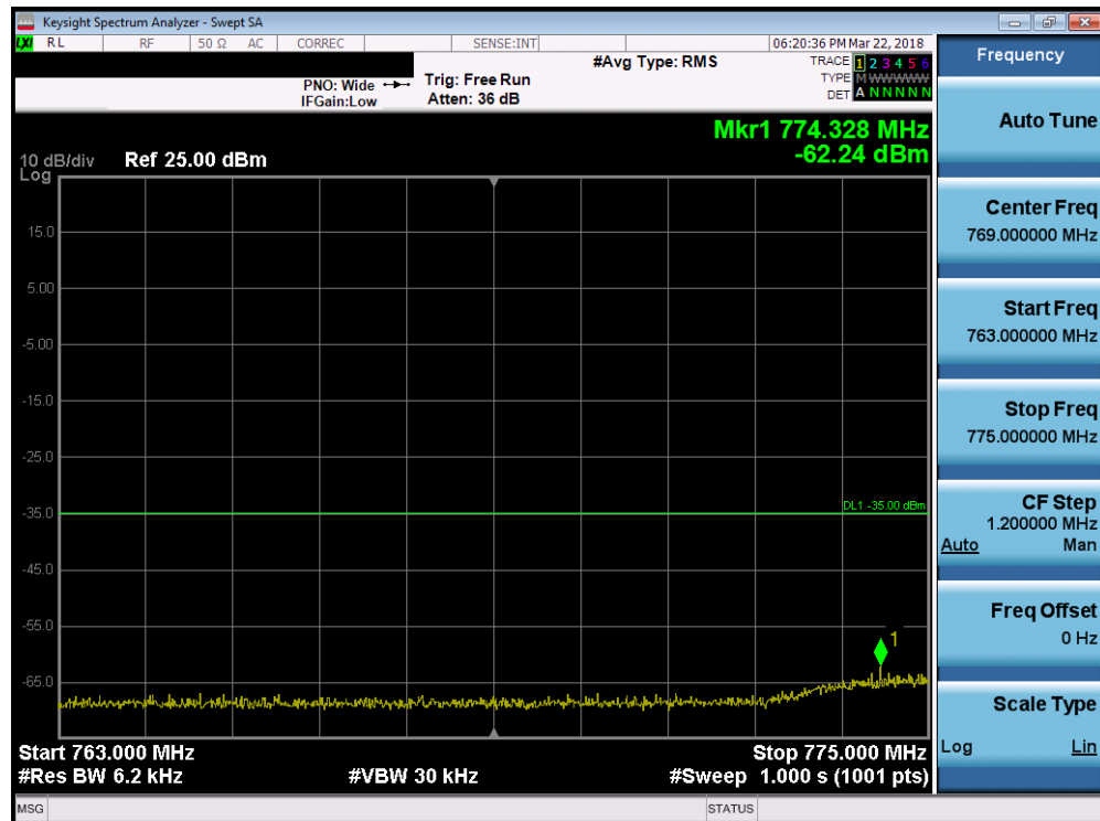
Plot 7-197. Lower Emission Mask Band Edge Plot (Band 13 - 5.0MHz QPSK - Full RB Configuration)
