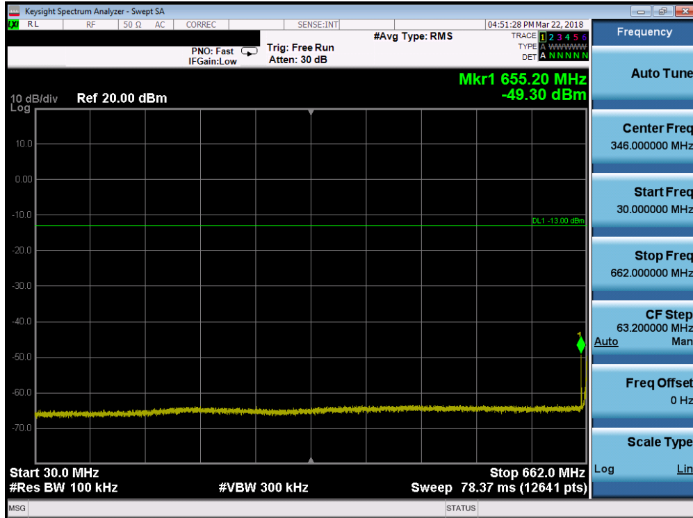
Plot 7-109. Conducted Spurious Plot (Band 71 - 20.0MHz QPSK - RB Size 1, RB Offset 0 - Low Channel)
