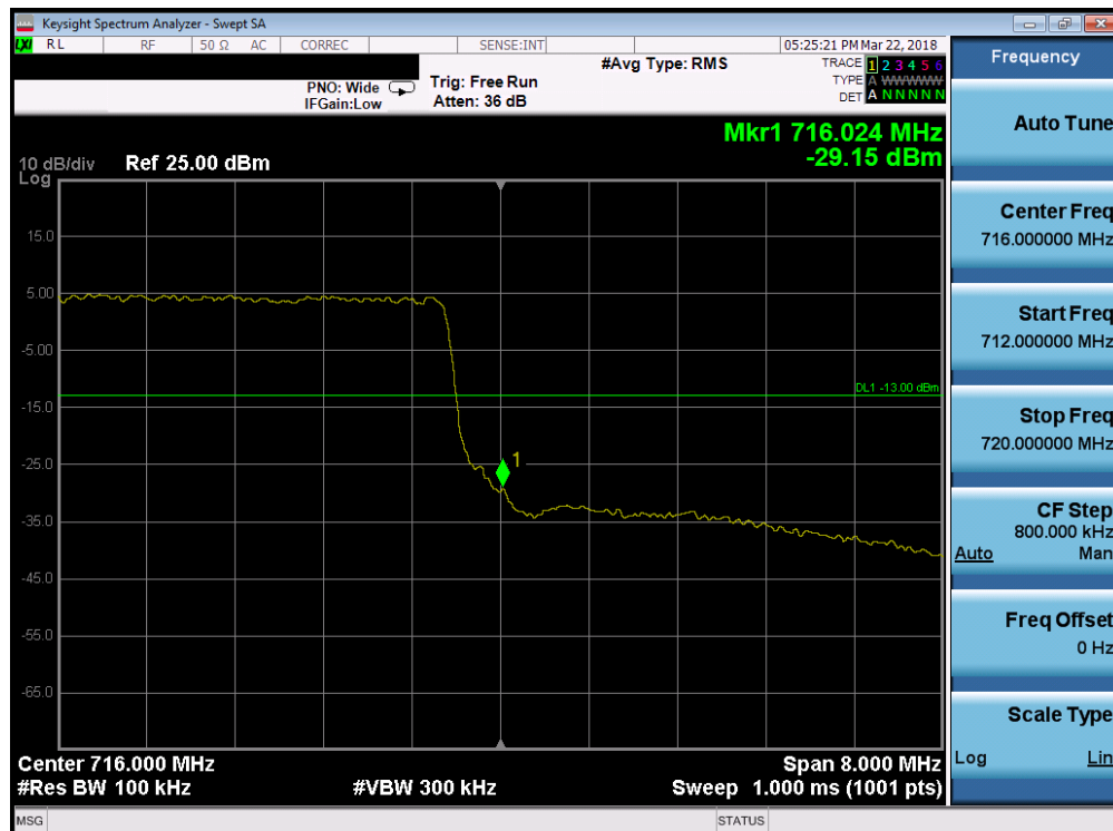
Plot 7-195. Upper Band Edge Plot (Band 12/17 - 10.0MHz QPSK - Full RB Configuration)
