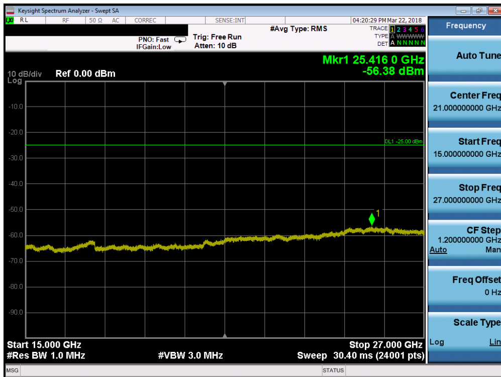
Plot 7-162. Conducted Spurious Plot (Band 7 - 5.0MHz QPSK - RB Size 1, RB Offset 0 - Low Channel)
