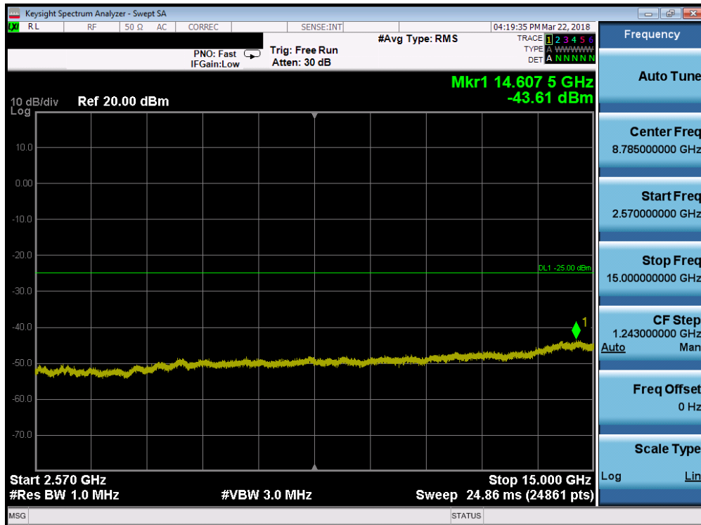
Plot 7-164. Conducted Spurious Plot (Band 7 - 5.0MHz QPSK - RB Size 1, RB Offset 0 - Mid Channel)
