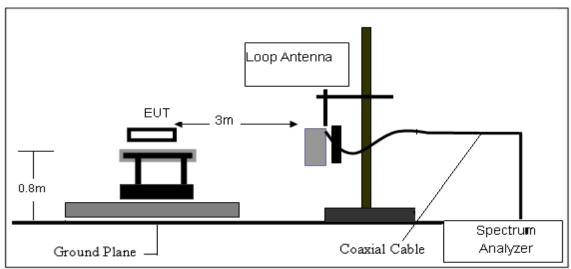
2. Radiated Emission Test-Up Frequency Below1GHz
