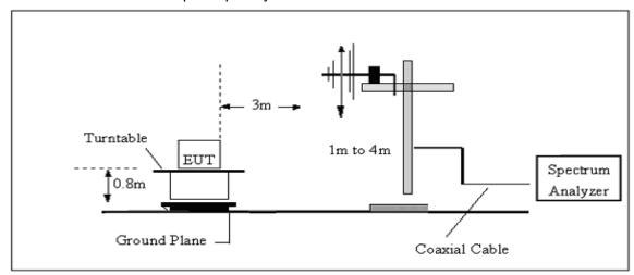
3. Radiated Emission Test-Up Frequency Above 1GHz
