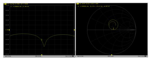
Dipole Verification Data> D3900V2, serial no. 1048
