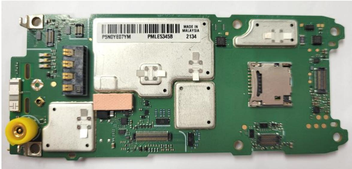
RF Board with Shields (Bottom), Model MXP600
