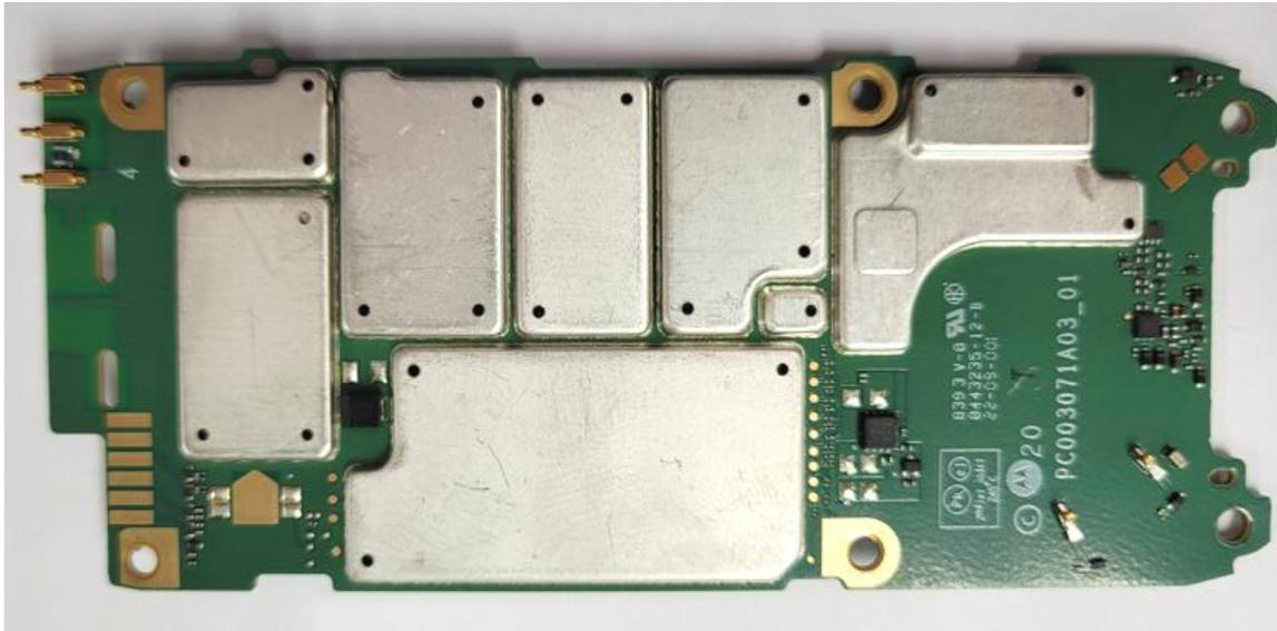
RF Board with Shields (Top), Model MXP600
