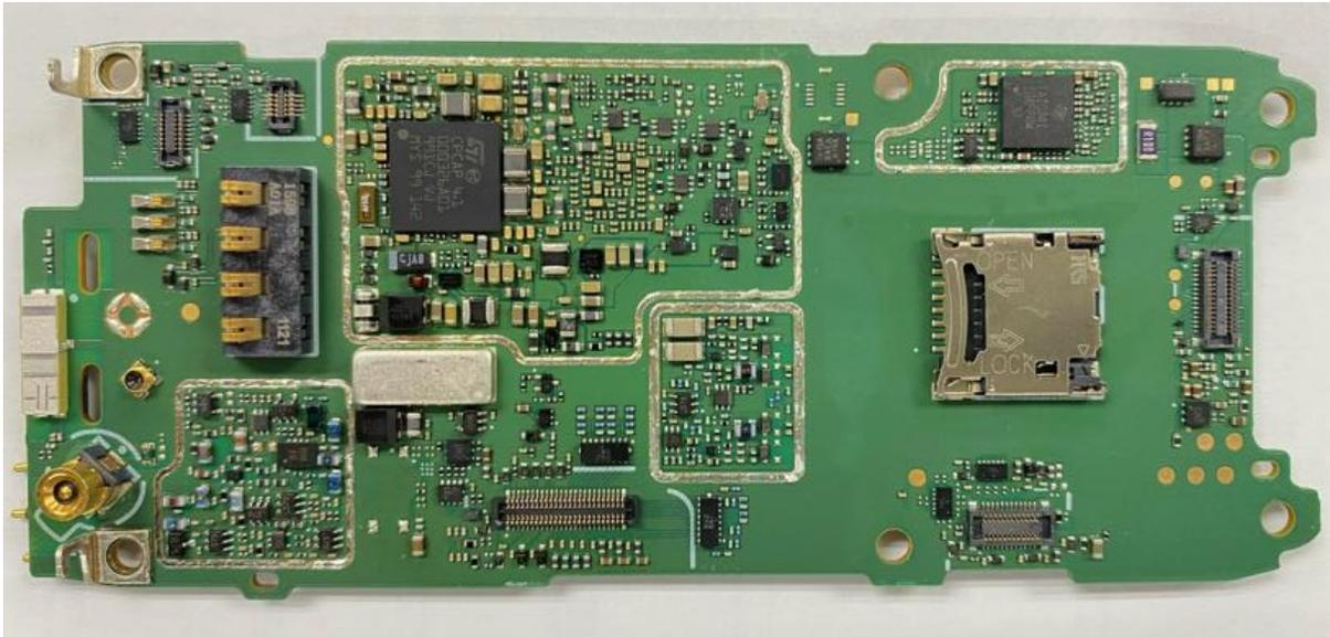
RF Board without Shields (Bottom), Model MXP600
