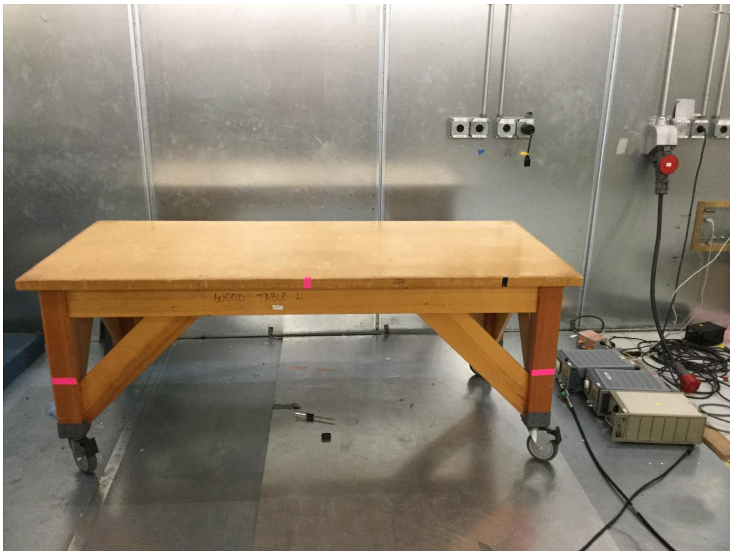
Figure 6 - Conducted Emissions Test Setup
