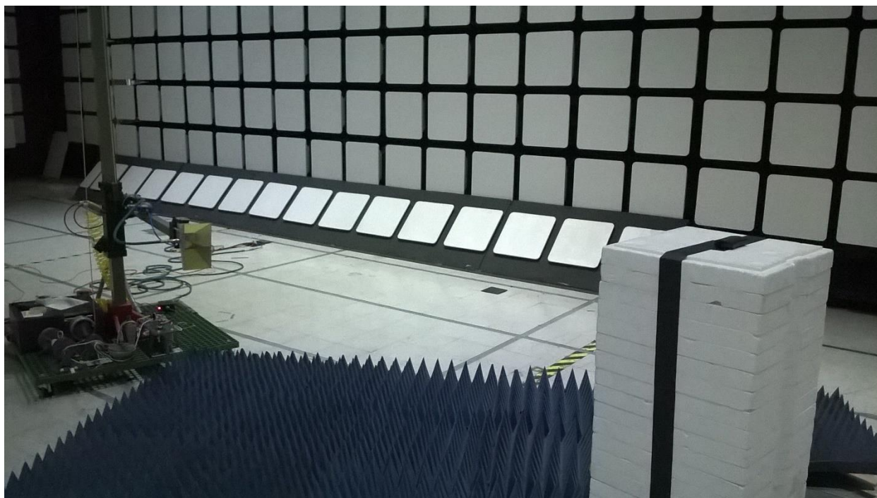
Figure 1 - Radiated Emissions Test Setup, 1 - 25 GHz, (EUT not shown)
