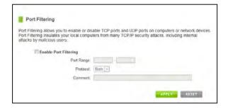
Hackers may sometimes scan for all open ports on your network as a method of hacking into your network. Port Filtering and other firewall features help to prevent this from happening.
