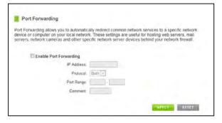
IP Address: The IP address of the device behind the Firewall that is being designated for Port Forwarding.
