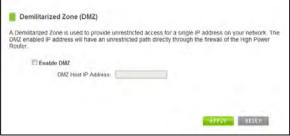
As a general safety rule, devices placed on the DMZ should not have any other network connections to any other devices.
