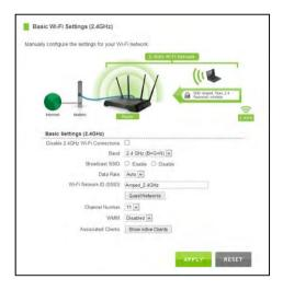
Wireless Network ID (SSID): The name of your 2.4GHz wireless network.
