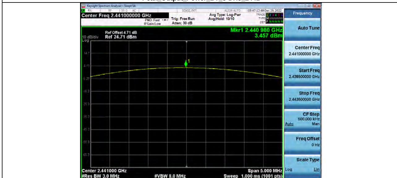
Peak Output Power_BT 3-DH5_2441
