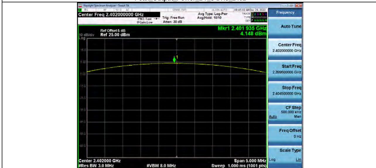
Peak Output Power_BT 3-DH5_2402
