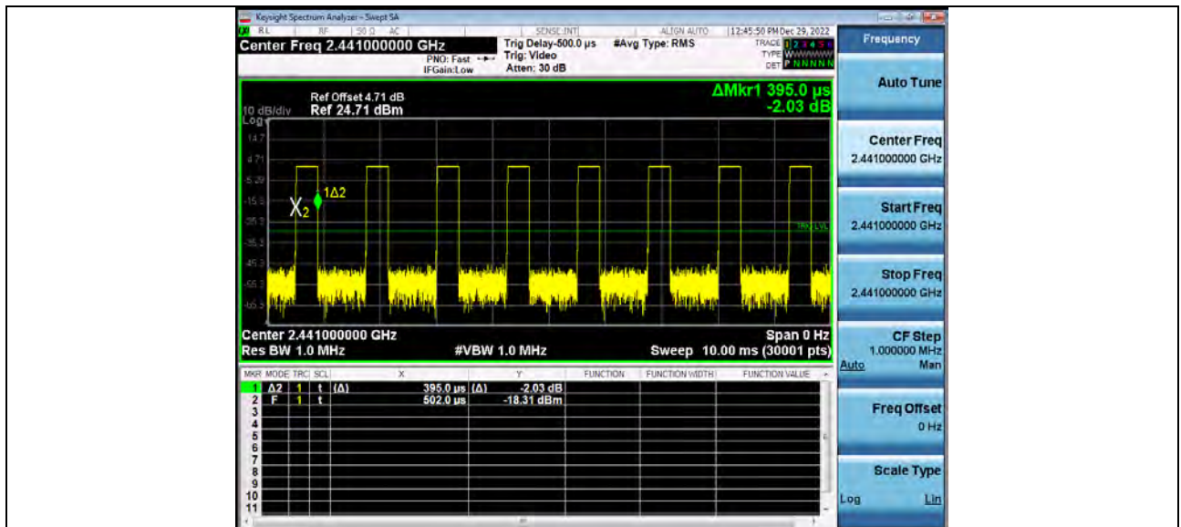
Dwell Time (Hopping) BT 2-DH5_2441_One_Burst_Time
