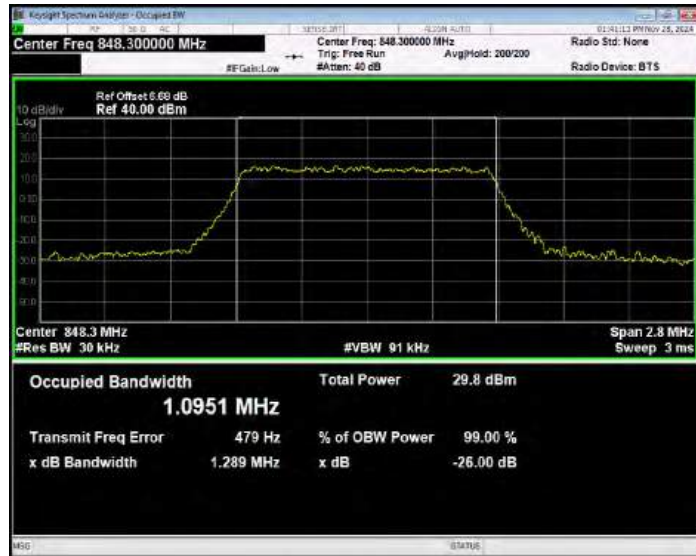
Band26(824-849) 16QAM BW=10MHz Channel=26840 RB Size=50 Position=#0
