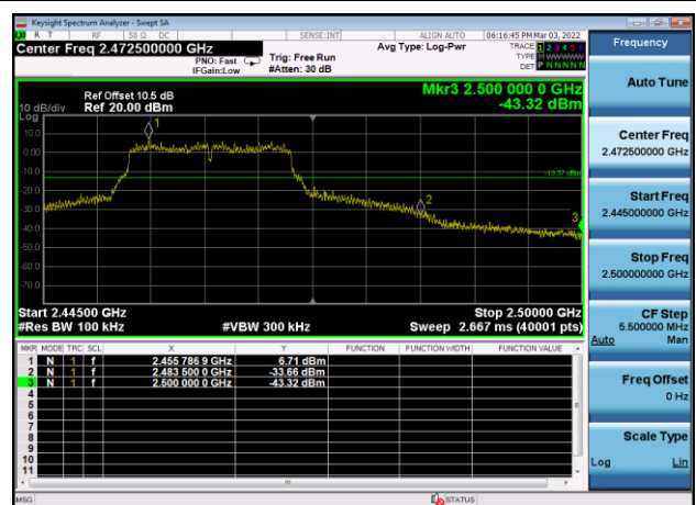
,Plot 2,Band Edge-802.11g,2462MHz ,Ant0
