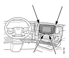
**9.** Move the infotainment system straight out and disconnect the connector and the antenna.
