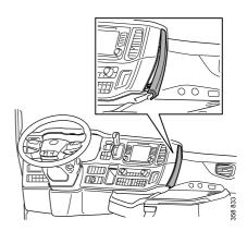
7. Fit the frame around the instrument cluster.
