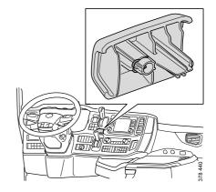
**8.** Fit the frame around the instrument cluster.
