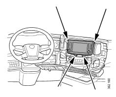
**11.** Move the infotainment system straight out and disconnect the connector and the antenna.
