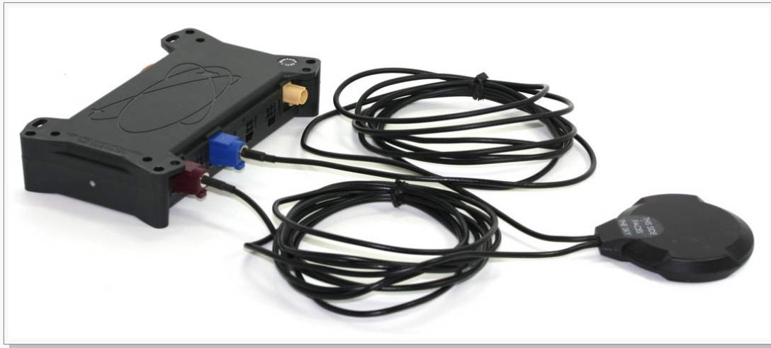
Figure 12: GSM/3G/GPS antenna ports
