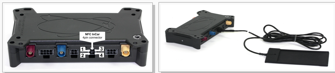
Figure 9: Pin assignments of 4-pin (2x2) connector and NFC InCar connection
