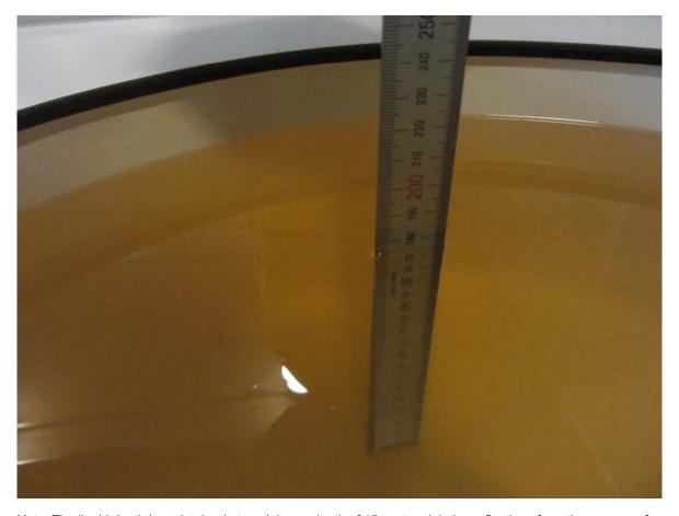
Note: The liquid depth is maintained at a minimum depth of 15 cm to minimize reflections from the upper surface.
